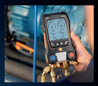
Thanks to Bluetooth® 5.0, the new digital manifolds with an extra-large display and robust safety housing are also suitable for wireless measurement. You save valuable time and avoid stress in the installation, maintenance and servicing of refrigeration systems and heat pumps. All important measurement programs are already stored in the system, as well as the right refrigerants for different plants.
